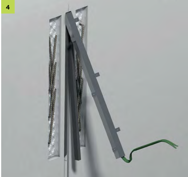
After casting the first section, remove the protective boxes of the FERBOX® rebend connectors, the protective boxes of the PENTAFLEX® Modul and the EPP filling strips.
