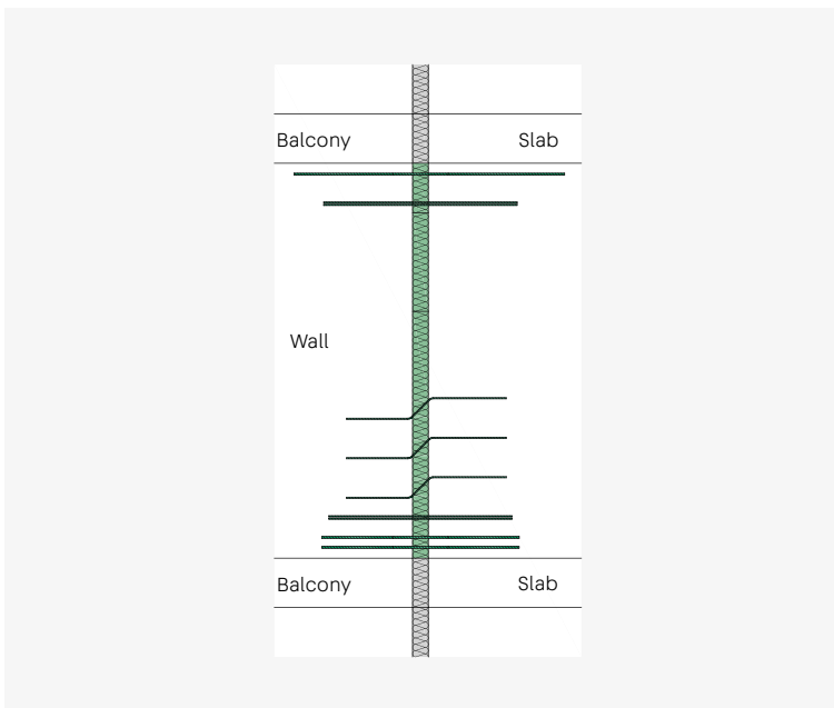
ISOPRO® IPTW – Installation cross-section with wall panel monolithically connected to the balcony slab
