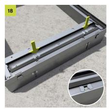
For stabilisation, a crossbeam is inserted and fastened to the end piece from above by two spring clamp fasteners. Screw in the M10 levelling bolts supplied before fixing the crossbeam.
