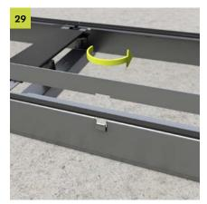
The adjusting strip can be set to 0 mm or 3 mm level. At 0 mm level, the notches in the adjusting strip are set flush with the side wall brackets. At 3 mm level, the notches are positioned next to the brackets. To do this, turn the adjusting strip horizontally by 180°.
