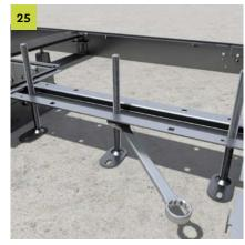
Secure levelling bases against loosening using lock nuts and shorten to the level of the crossbeam surface using a suitable tool.
