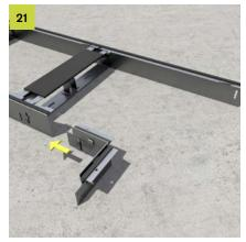
After shortening the duct side, screw the UBSFMAB mounting kit in place using holes and screws. If necessary, use a separately available template to mark the drill holes.
