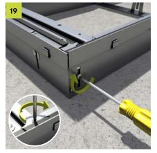
All screws on the duct side and the crossbeam must be tightened. Adjusting strips must be ordered separately.
