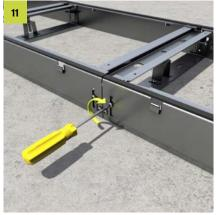
The base body and side walls are connected to each other by the upper screws on the duct wall. This fixes the set levelling height.
