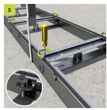
Adjust the height of the duct system using the M10 levelling screws, observing Fig. 4. Screed height according to the metre tear. The duct system may not be loaded.
