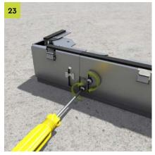
Screw the upper and bottom part of the outside corner to the side wall of the duct.
