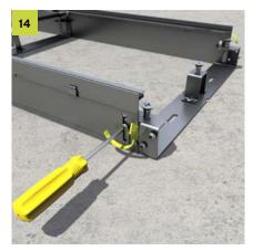
To mount the end piece, the levelling bracket and the associated screws must be removed.
