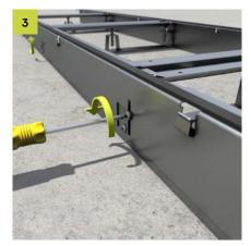
All upper screws must be loosened slightly on both duct walls. When delivered, these are tightened and provide stability during transport.
