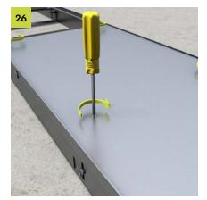
Align the blind cover on the duct and secure it from above using screws.
