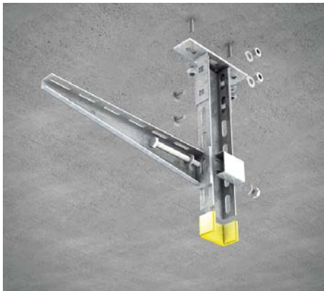
4 | Ceiling mounting with head plate BGU 57 and U-profile KHU 57 To install the BGU 57 use two dowels such as e.g. SD 10/10*. Mount the U-profile KHU 57 to the head plate BGU 57 using head screw set KLS 10x20*. Secure the bracket KW using KHUSS 57 support piece set. The protection cap SU 57* is fitted to the bracket bottom, if needed.
