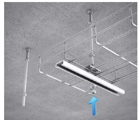
6 | Central suspension for wire mesh cable tray of up to 300 mm width Connect the central hanger GBAG 20/30 to the dowel using a hexagonal connector VM M8*. Mount the connector GV 30 as well as the profile rails with the wire-mesh cable tray inbetween both.
