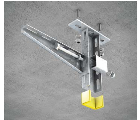
3 | Ceiling mounting with bracket support KDU 57 To install KDU 57 use two dowels such as e.g. SD 10/10*. Secure the bracket KW using KHUSS 57 support piece set. The protection cap SU 57* is fitted to the bracket bottom, if needed.
