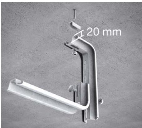
13 | Ceiling mounting with bracket support KSLW To install the KSLW use dowels such as e.g. SD 8/30*. The spacer KSL-SP must be positioned before the bracket support. Mount the bracket KSL using head screw FRS 8x20 and hexagonal nut SEMS 8.
