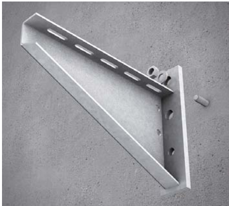
1 | Wall mounting with heavy bracket KWS To install KWS use dowels such as e.g. SD 12/10*. Please make sure to use the top drill hole to fixate the bracket.
