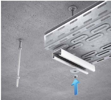
7 | Central suspension for cable trays of up to 300 mm width Connect the central hanger GBAR to the dowel using a hexagonal connector VM M10*. Dismount the profile rails and remount together with the cable trays.
