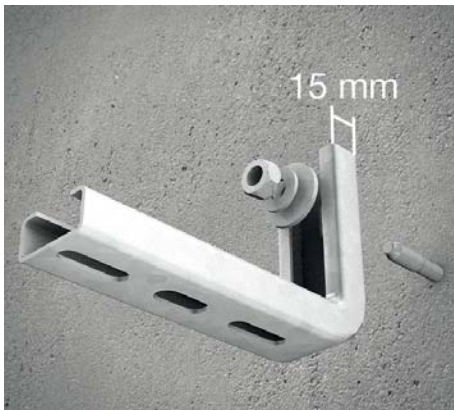
1 | Wall mounting with bracket KWLl To install the bracket KWLl use a dowel such as e.g. SD 8/30*. Please make sure to use the small washer of the dowel between the anchor nut and the large washer US 8x25*.
