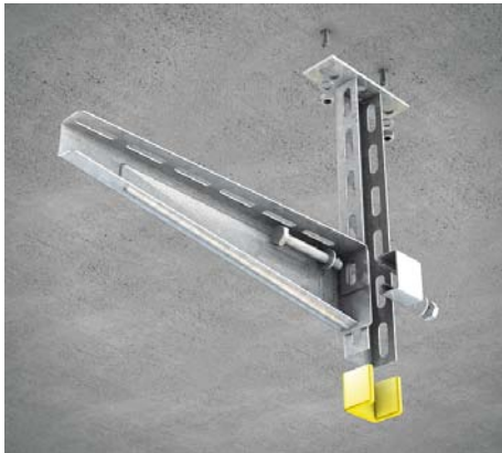
10 | Ceiling mounting with bracket support KDU 40 To install the KDU 40 use two dowels such as e.g. SD 8/10*. Secure the bracket KWF using KHUSS 40 support piece set. The protection cap SU 40* is fitted to the bracket bottom, if needed.
