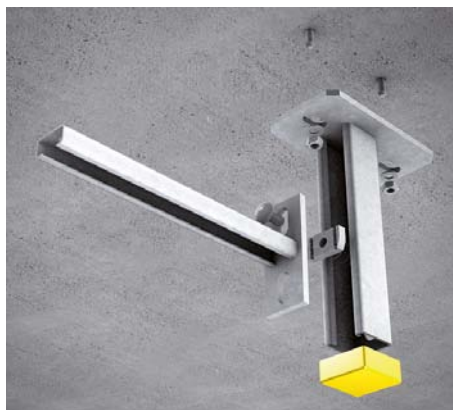
14 | Ceiling mounting with ceiling-fixed bracket KDAG 41 To install the KDAG 41 use two dowels such as e.g. SD 8/10*. Install the bracket KA 30 using full thread hexagonal head screw set SES 10x20*, channel spring nut AMF22 M10*. The protection cap SA* is fitted to the bracket bottom, if needed.
