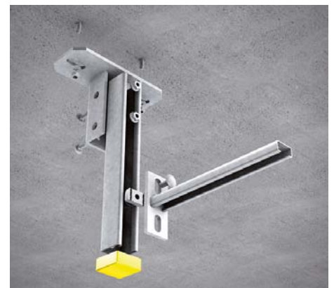
15 | Ceiling mounting with head plate BGA 41 and C-profile KHA 41 To install the BGA 41 together with the KHA 41 use two dowels such as e.g. SD 8/10*. Attach the C-profile to the KHA 41 by using head screw set KLS 10x20*. Fasten the bracket KA using full thread hexagonal head screw set SES 10x20* and channel nut spring AMF22 M10*. The protection cap SA* is fitted to the bracket bottom, if needed.
