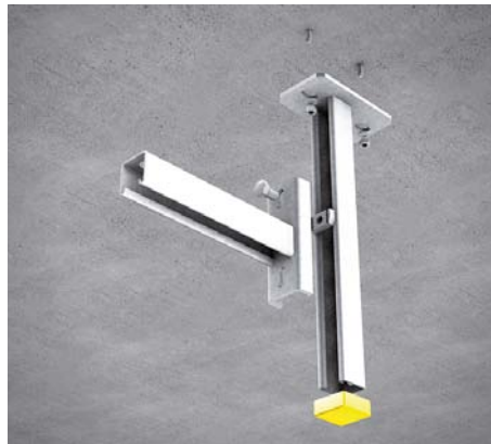
5 | Ceiling mounting with ceiling-fixed bracket KDAG 41 To install KDAG 41 use two dowels such as e.g. SD 10/10*. Then attach the bracket KA 41 using full thread hexagonal head screw set SES 10x20* and channel spring nut AMF22 M10*. The protection cap SU 57* is fitted to the bracket bottom, if needed.
