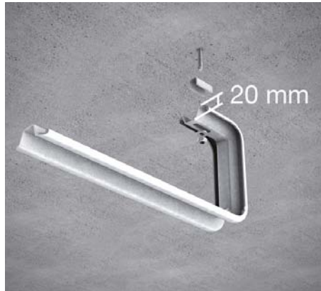
2 | Ceiling mounting with ceiling-fixed bracket DKSL To install DKSL use dowels such as e.g. SD 8/30*. The spacer KSL-SP must be positioned between the dowel and the bracket.
