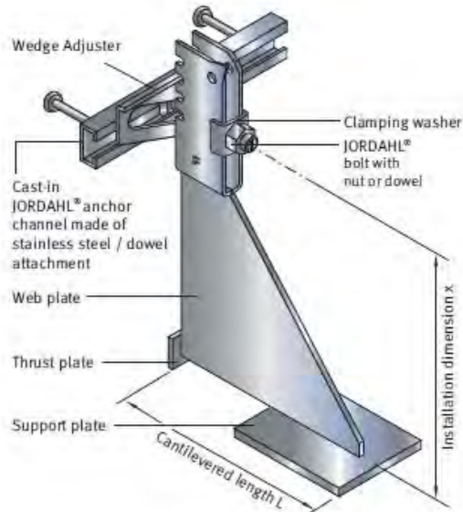
Figure 1: Brickwork support bracket with cast-in anchor channel
