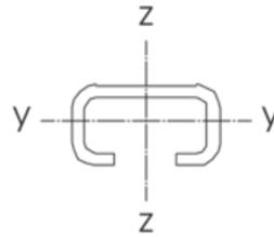
$$\begin{aligned}W_y &= 0.30 \text{ cm}^3 \\W_z &= 0.83 \text{ cm}^3 \\I_y &= 0.25 \text{ cm}^4 \\I_z &= 1.25 \text{ cm}^4\end{aligned}$$
