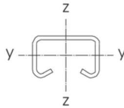
$$\begin{aligned}W_y &= 2.31 \text{ cm}^3 \\W_z &= 5.40 \text{ cm}^3 \\I_y &= 3.77 \text{ cm}^4 \\I_z &= 13.49 \text{ cm}^4\end{aligned}$$
