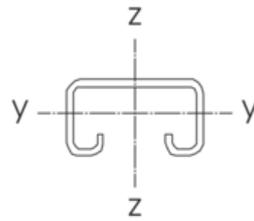
$$\begin{aligned}W_y &= 1.10 \text{ cm}^3 \\W_z &= 2.25 \text{ cm}^3 \\I_y &= 1.34 \text{ cm}^4 \\I_z &= 4.32 \text{ cm}^4\end{aligned}$$
