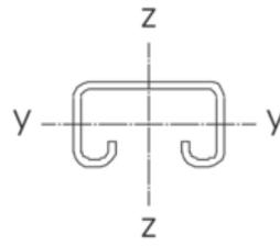
$$\begin{aligned}W_y &= 0.90 \text{ cm}^3 \\W_z &= 1.75 \text{ cm}^3 \\I_y &= 1.10 \text{ cm}^4 \\I_z &= 3.46 \text{ cm}^4\end{aligned}$$
