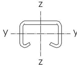
$$\begin{aligned}W_y &= 1.25 \text{ cm}^3 \\W_z &= 2.85 \text{ cm}^3 \\I_y &= 1.70 \text{ cm}^4 \\I_z &= 5.62 \text{ cm}^4\end{aligned}$$
