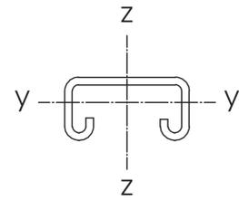
$$\begin{aligned}W_y &= 0.92 \text{ cm}^3 \\W_z &= 2.56 \text{ cm}^3 \\I_y &= 1.02 \text{ cm}^4 \\I_z &= 5.25 \text{ cm}^4\end{aligned}$$
