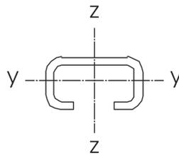
$$\begin{aligned}W_y &= 0.32 \text{ cm}^3 \\W_z &= 0.83 \text{ cm}^3 \\I_y &= 0.30 \text{ cm}^4 \\I_z &= 1.26 \text{ cm}^4\end{aligned}$$
