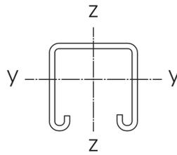
$$\begin{aligned} W &= 3.19 \text{ cm}^3 \\ W_y &= 4.50 \text{ cm}^3 \\ I_y &= 7.31 \text{ cm}^4 \\ I_z &= 9.22 \text{ cm}^4 \end{aligned}$$
