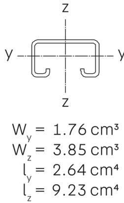
$$\begin{aligned} W_y &= 1.76 \text{ cm}^3 \\ W_z &= 3.85 \text{ cm}^3 \\ I_y &= 2.64 \text{ cm}^4 \\ I_z &= 9.23 \text{ cm}^4 \end{aligned}$$
