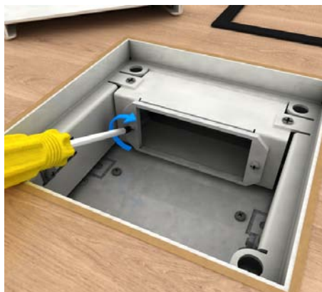
14 | Installation devices Snap the installation components into plug-in board (UGEE3) from the front, mount the connection line and screw the entire element to the device carrier.
