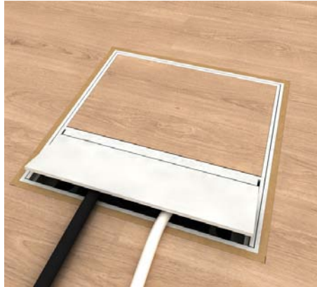
8 | Single outlet Insert the rubber seal and cartridge cover. Open the cover and pull the cable out through the cable outlet. For dry floors, install the cartridge installation unit with cable outlet. Pay attention to equipotential bonding.
