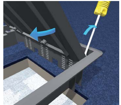
3 | Remove hinged cover Open cover completely, pull firmly forward at the right side and loosen from hinge joint with a screwdriver.
