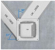
Using the hollow space floor box UBDHB250 When using the hollow space floor box UBDHB250, the screed-covered duct maximal can be inserted with a maximum angle of 51° without affecting the function. Cutting positions must be deburred and galvanised with cold zinc.
