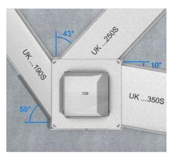
Using the hollow space floor box UBDHB350 When using the hollow space floor box UBDHB350, the screed-covered duct maximal can be inserted with a maximum angle of 55° without affecting the function. Cutting positions must be deburred and galvanised with cold zinc.
