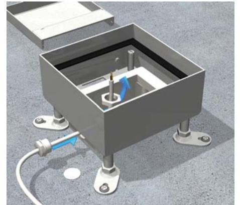
3 | Cable entry For the cable entry use a tool to break the lateral perforation out of the frame and complete with strain relief.
