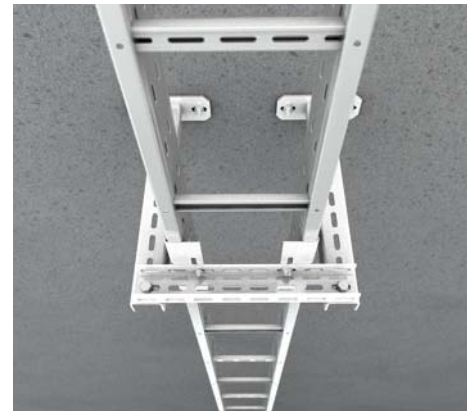
6 | Profiles Pendant suspension from profiles (e.g. KHU 60) with crossbeam and side-rail support (WPHS-K) are anchored to concrete ceiling.
