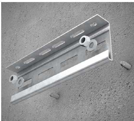
4 | Wall mounting with bracket KWW To install the bracket KWW use a dowel such as e.g. SD 8/10*. Please use the outer slots of the profile to fixate the bracket.
