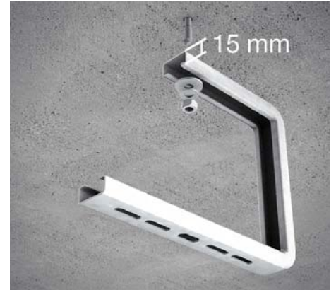
9 | Ceiling mounting with ceiling-fixed bracket DB To install the bracket DB use dowels such as e.g. SD 8/30*. Please make sure to use the small washer of the dowel between the anchor nut and the large washer US 8x25*.
