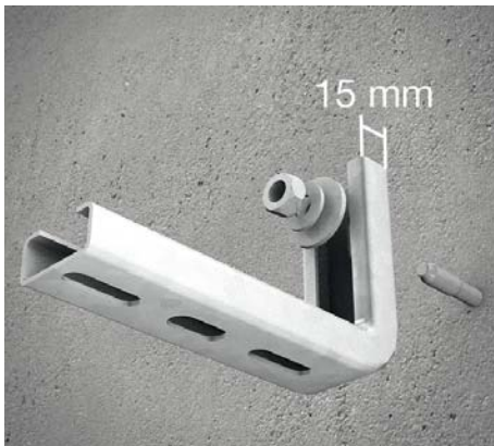
1 | Wall mounting with bracket KWL To install the bracket KWL use a dowel such as e.g. SD 8/30*. Please make sure to use the small washer of the dowel between the anchor nut and the large washer US 8x25*.
