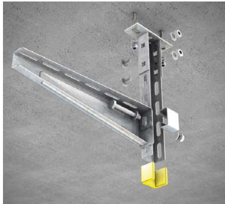
11 | Ceiling mounting with head plate BGU 40 and U-profile KHU 40 To install the BGU 40 use two dowels such as e.g. SD 8/10*. Mount the U-profile KHU 40 to the head plate BGU 40 using head screw set KLS 10x20*. Secure the bracket KWF using KHUSS 40 support piece set. The protection cap SU 40* is fitted to the bracket bottom, if needed.
