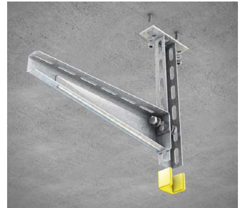
12 | Ceiling mounting with bracket support KDU 40 at reduced load - without supporting piece KHUSS 40 To install the KDU 40 use two dowels such as e.g. SD 8/10*. The bracket KWF is mounted with full thread hexagonal head screw 10x20* and two washers US 10x21* onto bracket support. The protection cap SU 40* is fitted to the bracket bottom, if needed.
