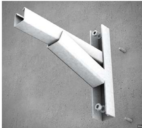
2 | Wall mounting with heavy bracket KWSS To install KWSS use dowels such as e.g. SD 12/10*. Please make sure to use the top and bottom drill holes to fixate the bracket.
