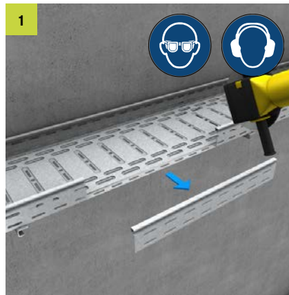
Tray extension angle (RAE) Cut out the side rail of the cable tray flush with the bottom in width B = connecting cable tray width + 120 mm, deburr and cold-galvanise.
