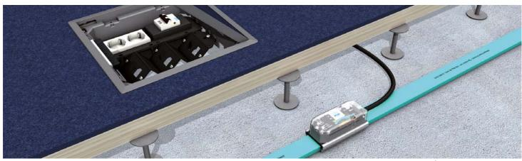
Pre-tailored device cups with a snap-in device socket, pre-wired sockets, a flat conductor adapter connected to a 2 m/3 m connecting cable (3 x 4 mm<sup>2</sup>) and 16 A FI/LS switch. Including all covers and assembly materials. To be latched into a round or square installation unit. For direct connection to 5 x 10 mm<sup>2</sup> flat conductors. Fuse of 50 A.
