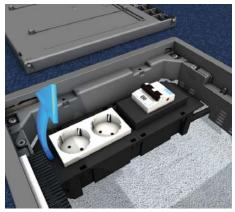
**6** | Install device cup Insert the pre-tailored device cups as deeply as possible into the lock-in leads of the installation unit. Leave the central device cup slot empty to install data technology later on.
