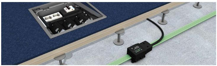
Pre-tailored device cups with a snap-in device socket, pre-wired sockets, a flat conductor adapter connected to a 2 m/3 m connecting cable (3 x 4 mm<sup>2</sup>) and 10 A FI/LS switch. Including all covers and assembly materials. To be latched into a round or square installation unit. For direct connection to 5 x 2.5 mm<sup>2</sup> / 4 mm<sup>2</sup> flat conductors. Fuse of 20 A.
