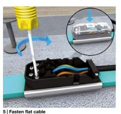
Fasten flat cable to the connector module with screws, then place body onto the cover. Pay attention to the correct torque (1,2 - 1,4 Nm)! If the cover does not close completely, not all screws have been tightened correctly!
