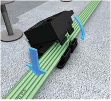
**3** | Insert the flat cable Insert the flat cable into the coded base plate. Keep in mind the correct installation direction for the outgoing direction of the connector. Afterwards close the connection module.
