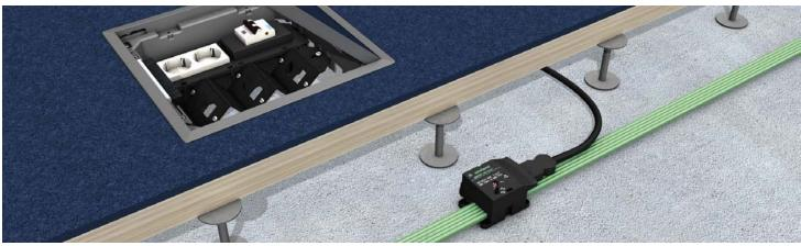
Pre-tailored device cups with a snap-in device socket, pre-wired sockets, a flat conductor adapter connected to a 2 m/3 m connecting cable (3 x 2.5 mm<sup>2</sup>) with 3-pole plug and 6 A FI/LS switch. Including all covers and assembly materials. To be latched into a round or square installation unit. For direct connection to 5 x 2.5 mm<sup>2</sup> / 4 mm<sup>2</sup> flat conductors. Fuse of 20 A.
