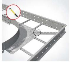
**16 | Additional rung to corner attachment** Screw the additional rung with the corner attachment by using screws (FKS 6x20) and channel nuts (AMA 18 M6).
