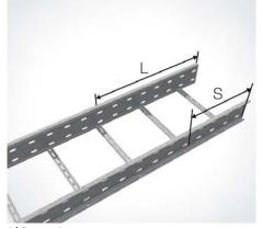
**2** | Separating cut ranges Add 150 mm to the ladder width to get the area of the removable rungs (S). Add 520 mm to the ladder width to get the area of the removable side beams (L).
