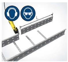
**4 | Separat the side beams** Remove completely the side beams from the rungs of both wide-span cable ladders.
