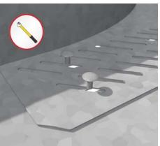
**9 | Assemble the corner attachment** Lead the screws from top to down and screw them from the bottom with a nut (SEMS M6).
