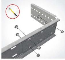
**7 | Bend the corner connector** Bend the corner connector centrally up to 90 degrees and screw it with the outside of the side beam using three screws (KLS 10x20).
