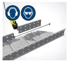
**4 | Separat beams and floor plates** Separat the side beams from the remaining floor plate shown in area L and remove them completely.
