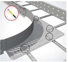
**11 | Screw the rungs** Screw all four rungs with the corner attachment by using two screws (FRS 6x25) per rung.
