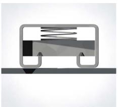
**14 | Complete an additional rung** Position the channel nut (AMF 18 M6) in the end of a rung and lay it on the beam support (WHPS) with the open profile side.
