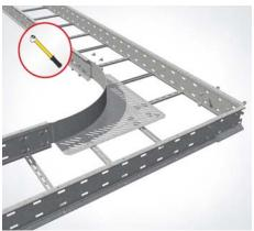
**9** | Assemble the attachment tray Screw the attachment ladder with the corner attachment through the corner connector by using four screws (KLS 10x20) per crossover.
