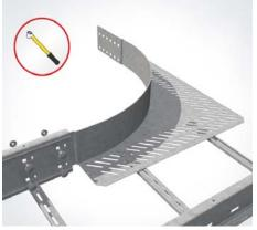
**6** | Assemble the corner Screw the connector of the corner connector with the outside of the side beams by using four screws (KLS 10x20).
