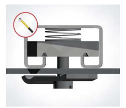
**15** | Assemble the additional rung Screw the screw (FKS 6x20) and its clamping piece (KLU) with the beam support (WHPS) and the channel nut (AMF18 M6).
