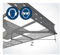
**12 | Create an additional rung** Cut the profile (KHA) to the required dimensions: ladder width added with 200 mm.
