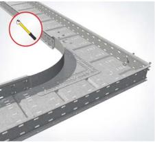
**8 | Complete the corner connector** Position the side beam support (WHPS) close to the corner and screw it with the side beam by using the connector (WPVH) and a screw (KLS 10x20).
