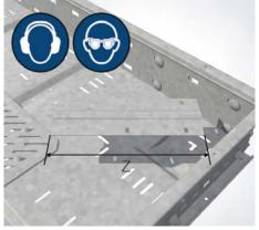
**11 | Separate the connection plate** Cut the connection panel (VB-BS) to the required length Z (tray width less 100 mm).
