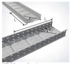
**1 | Mark the separating cuts** Select the inner side beams of the direction change for marking the separating cuts. The inner side beams are removed in area L.
