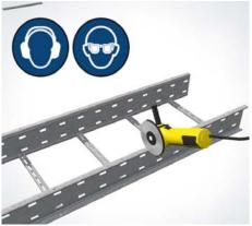
**17** | Separate and cut If cutting or separating is needed, pay attention to the health and safety protection at the workplace.
