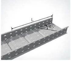
**2** | Separating cut ranges Add 520 mm to the ladder width to get the area of the removable side beams (L). Use mitre cuts of the track ends.
