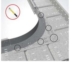
**10 | Screw the corner attachment** Screw the corner attachment with five screws (FRSV 6x16) per hole series (in total ten screws).
