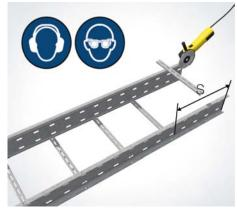
**3 | Separat the rungs** Remove completely all frames from both tracks in area S.
