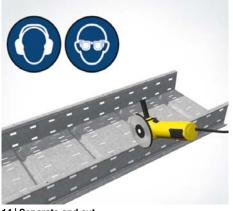
**14 | Separate and cut** If cutting or separating is needed, pay attention to the health and safety protection at the workplace.
