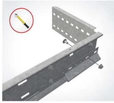
8 | Complete the corner connector Position the side beam support close to the corner and screw it with the side beam by using the connector (WPVH) and one screw (KLS 10x20).
