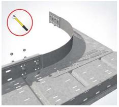
**6** | Assemble the corner attachment Screw the connector of the corner attachment with the outside of the side beams by using four screws (KLS 10x20).
