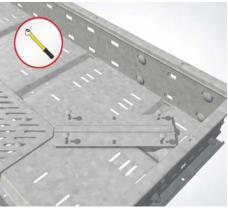
12 | Assemble the connection plate In the mitre cut area, screw the connection plate (VB-BS) with the cable tray bottom using four screws (FRSV 6x16) and nuts (SEMS M6).
