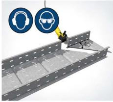
**3 | Mitre cut in floor plate** Use mitre cuts in 45 degrees at the end of the widespan cable trays and the floor plate.
