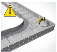
**13 | Assemble the connection plate** If needed, drill missing holes with  $\emptyset = 7$  mm in the cable tray according to the connection plate.
