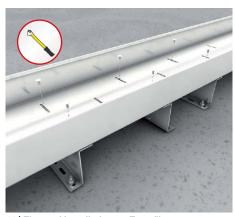
**44 | Elevated installation on Z profile** The Z profile is used for installation at a raised level. For this purpose, select the appropriate fastener (Dmax = 8mm) for the base provided. Mark the drilling holes and drill directly. Ensure that the strap on the floor is arranged on alternate sides and the maximum distance between the supports is not exceeded. After drilling, remove the bore dust completely and mount the fastener. Screw-fit the floor duct.
