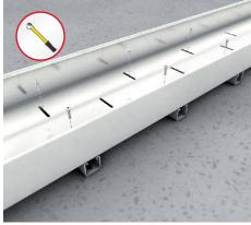
**43 | Continued installation on C profile** To mount the fastener, use channel nuts with M6 threading and insert in the profile. Screw-fit the floor duct with a M6 flat head screw.
