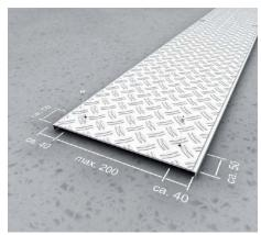
37 | Note the following: when shortening the floor duct cover with chequered plate
