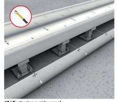
**47 | Fastening a side panel** Select a side panel with an appropriate lateral height. Use a floor bracket or floor duct bracket with an appropriate mounting plane. Hold the side panel and fasten with appropriate connecting elements.
