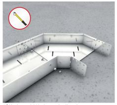
**5** | Horizontal 90° change in direction If there is a 90° change in direction, push the floor duct bend into the side beams of the floor duct using the pre-assembled couplers, and secure it using two clamping screws per side beam.
