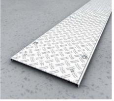
**20 | Floor duct cover with a chequered plate** In this model, an aluminium chequered plate of antislip class R10 (DIN 51130) is riveted on the floor duct covers using turning bolts.
