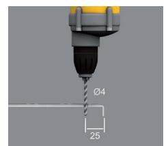
**33 | Preliminary drilling** A hole with D = 4 mm each is pre-drilled for the floor duct cover with chequered plate.
