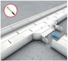
**12 | Floor duct attachment branch-piece** Slide the floor duct attachment branch-piece on the floor duct to be connected and secure it using 2 clamping screws per side beam.
