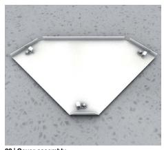
22 | Cover assembly The covers are fitted with turning bolts. Before mounting the covers on the floor duct, ensure that the turning bolts are parallel to the edge of the cover and aligned to the left.
