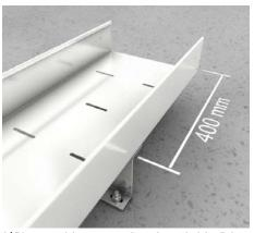
**3** | Distance of the supports from the end of the fitting The maximum distance between the last support and the end of the duct piece should not exceed 400 mm.
