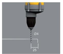
**27 | Preliminary drilling** A hole with D = 4mm each is pre-drilled for assembling turning bolts.
