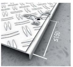
**32 | Positioning of the turning bolts** Floor duct covers with an aluminium chequered plate require preliminary drilling for the new turning bolt. The turning bolts can be pre-machined with the step drill.
