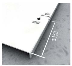
**26 | Positioning of the turning bolts** Floor duct covers without anti-slip structure require preliminary drilling for new turning bolts.
