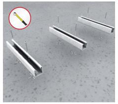
**42 | Elevated installation on C profile** C profile is used for installation at a raised level. For this purpose, select the appropriate fastener (Dmax = 8mm) for the base provided. Then lay the C profile with the closed side on the floor. In doing so, ensure that the maximum distance between the supports is not exceeded. Mark the drilling position through the openings or drill directly. After drilling, remove the bore dust completely and mount the fastener.
