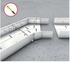
**6 | Horizontal 45° change in direction** For a 45° change in direction, use the 45° degree floor duct bend and secure it using 2 clamping screws per side beam.
