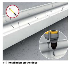
Installation can be carried out directly on the floor. For this purpose, select the appropriate fastener (Dmax = 6mm) for the base provided. Then lay the floor duct on the floor. Mark the drilling position through the openings on the bottom plate or drill it directly. After drilling, remove the bore dust completely and mount the fastener.
