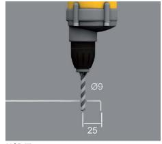
**28** | **Drilling** After preliminary drilling, the corresponding holes are drilled with D= 9mm and deburred.
