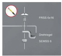
25 | Assembly of turning bolts
