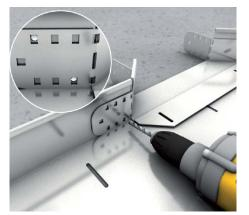
**11** | Floor duct attachment branch-piece On the section, drill two holes on each side beam for securing the screws. Drill  $2 \times D = 6.5$ mm through the holes in the pre-assembled couplers, as shown.
