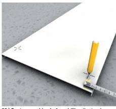
35 | Centre-punching before drilling the turning bolt position
