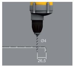
**30 | Preliminary drilling** A hole with D = 4mm each is pre-drilled for the floor duct cover with chequered plate.
