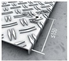
**29 | Positioning of the turning bolts** Floor duct covers with an anti-slip structure require preliminary drilling for new turning bolts. The turning bolts can be pre-machined with a step drill.
