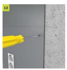
Secure the cover to the base body with a screw. If the cover is mounted offset on the base body, a new hole (Ø 4.5 mm) must be drilled in the base body.
