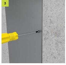
Unscrew the mounting cover from the base body using a Phillips screwdriver.
