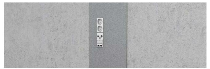
Flush-wall duct system WANDA consisting of base body, installation devices and covers. The base body, which is already integrated into the concrete, is 2500 mm long and is supplied with mounting channels and mounting covers. The basic body is completed on site with two project-specific covers (1250 mm) and freely selectable installation devices.
