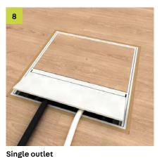
Insert the rubber seal and cartridge cover. Open the cover and pull the cable out through the cable outlet. For dry floors, install the cartridge installation unit with cable outlet. Pay attention to equipotential bonding.
