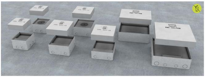
Square compact single outlet with dimensions  $125 \times 125$  mm,  $160 \times 160$  mm,  $184 \times 258$  mm and  $258 \times 258$  mm for screed installation in dry and wet floors. The floor box, the stainless steel unit and the shuttering unit are included in delivery. For parquet and stone flooring with a thickness of 12/22 mm and height-adjustable between 80 - 95 or 90 - 135 mm.
