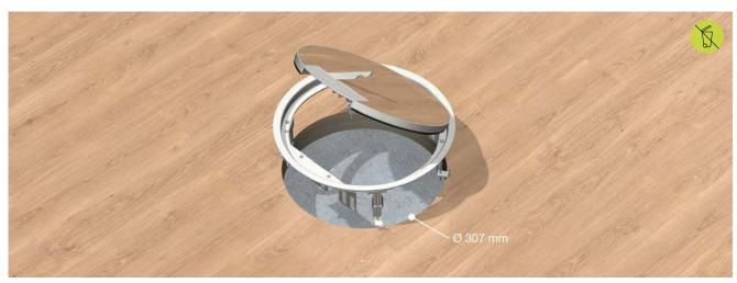
Cartridge installation units with a protective floor covering frame made out of stainless steel, round, with an outside diameter = 330 mm, for hollow space or false floors, with a clamping range from 40 to 80 mm. Usable for floor coverings with a thickness of 12 mm.
