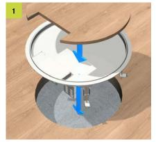
Cartridge installation unit Insert the cartridge installation unit (UEKDD R E) which is usable for up to three mounting boxes in the floor opening.
