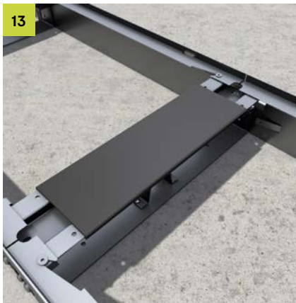
13 The impact sound profile is clamped centrally on the crossbeam. The drill holes for fixing the covers must not be covered.
