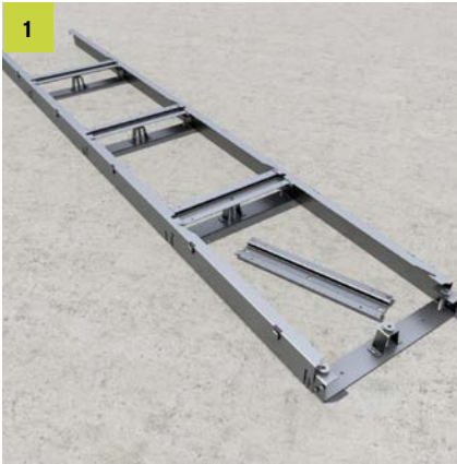
1 Screed-flush duct UBSF, consisting of the base body with four levelling brackets, centre support, three screwed crossbeams and one loose crossbeam including screws.
