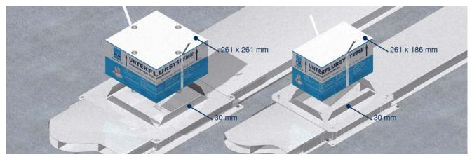
Hollow space floor box for quadrangular installation units 258 x 258 mm or 258 x 184 mm and underfloor ducts of up to 250 or 350 mm width with the heights 28/38/48 mm. Comply with minimum screed covering of 35 mm.
