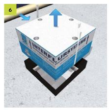
Removal of shuttering unit Remove shuttering unit with the release cord from the hardened screed. Process floor cover to the cleaned installation opening (261 x 261 mm, 261 x 186 mm).
