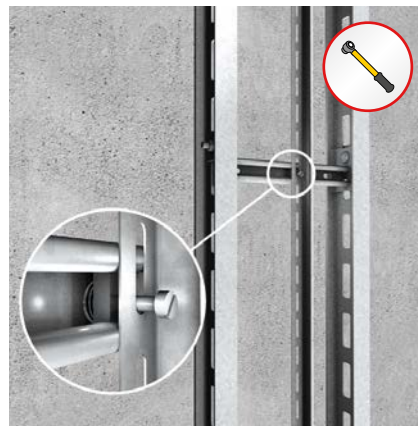
Separating strip STR 50 Screw the separating strip (STR 50) three times with a channel nut with spring (AMF18 M6) and slotted cylinder head screw (FKS 6x20), at the first and last rung as well as centrally.
