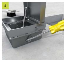
Remove the perforation on the side walls of the floor socket and insert the empty conduit.
