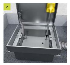
The horizontal alignment and height adjustment of the floor socket is done via the four adjusting screws. If necessary, the floor socket can be fixed to the subfloor.
