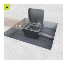
Insert the floor socket into the cavity. Ensure that the floor socket is aligned at finished floor level.
