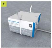
Fix the empty pipes to the aligned formwork body. Before placing the screed, fix the formwork body to the unfinished floor and secure it against floating.
