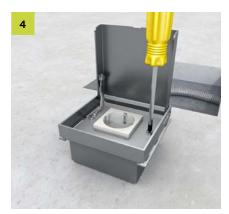
Detach the cover plate and the earth wire from the frame of the floor socket.
