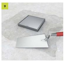
Before placing the mortar, check the position of the floor socket. Apply the mortar without air pockets, if necessary mask the gap between the frame and the cover.
