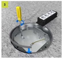
Adjust the installation frame to the height of the Adjust to the height of the finished floor. Seal the expansion joint all around with cork or sealing compound.
