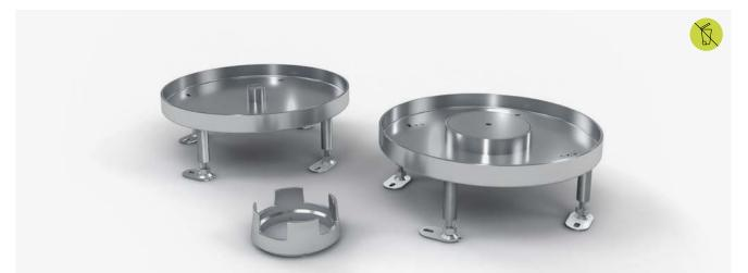
Round cartridge units with butt edge made of stainless steel. Outer diameter of 305 mm as dummy and tube cassette unit. Suitable for floor coverings with a thickness of 22 mm and for cleaning with floor cleaning machines. Height-adjustable from 110 to 165 mm.
