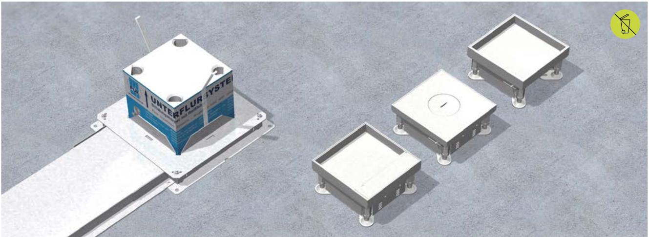
Quadrangular single outlets with external dimension of 160 x 160 mm for the integration of up to two installation devices of 45 x 45 mm for fixture in hollow space floor boxes.
