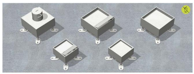
Quadrangular single outlets with outer measurements of 115  $\times$  115 mm for the integration of up to two installation devices of 45  $\times$  45 mm for direct screed mounting.
