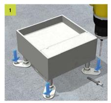
**Fixating**Mount the four levelling legs onto the rough concrete ceiling with nail plugs.
