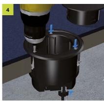
Fasten strain relief and frame Insert the strain relieves from below and secure cable. Tighten claws with phillips head screws.
