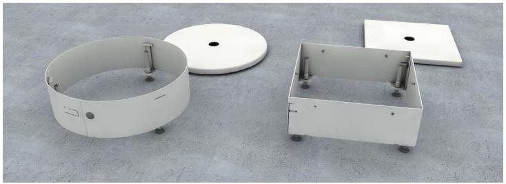
Grindable shuttering unit (UNSKH), round and quadrangular, height-adjustable between 96 - 155 mm. Installation dimensions Ø 308 mm (round) and 261 x 261 mm (quadrangular). For grindable cast-asphalt and screed floors, consisting of a foldable unit, levelling bases and a grindable cover.
