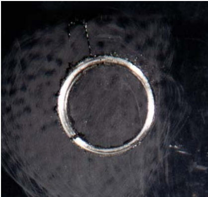
Punch tear test shows little to no detachment.
