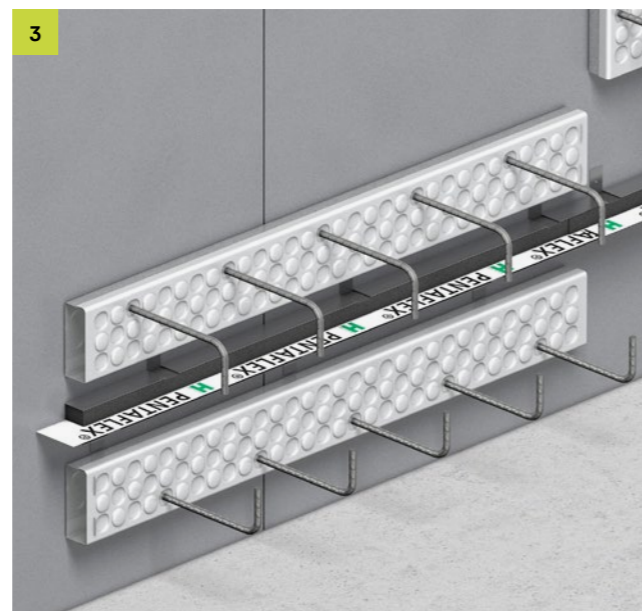
3 Next to the PENTAFLEX® Modul, nail two single-row FERBOX® rebend connectors to the formwork
