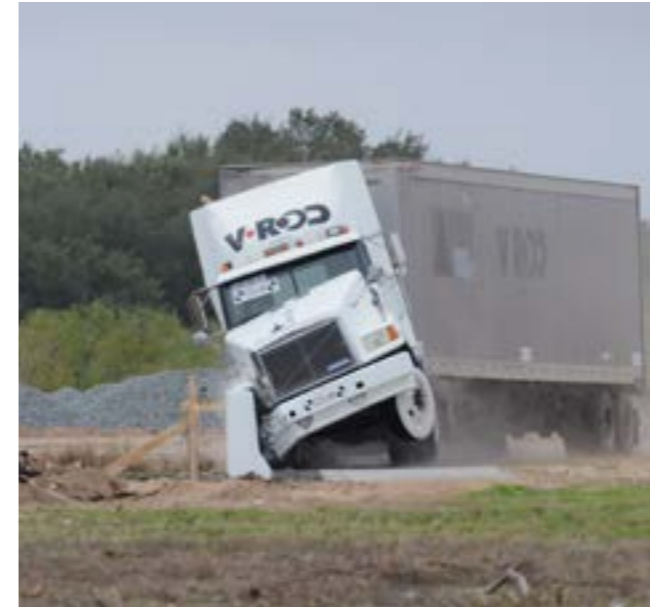
Impact test of a 36,000-kg truck travelling at 80 km/h against a standard crash barrier reinforced with FIBERNOX® V-ROD
