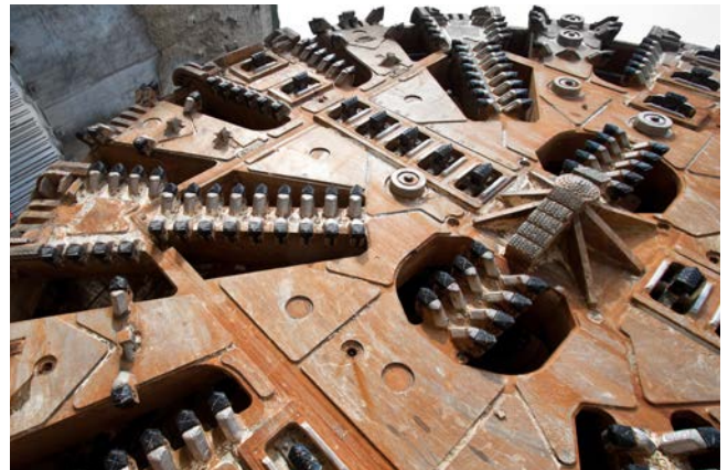
Thanks to modern tunnel boring machines, tunnel tubes with a diameter of more than 17.5 metres can be produced.
