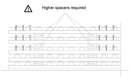
JORDAHL punching shear reinforcement JDA
