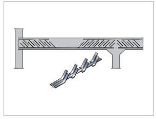
The Kahn steel reinforcement system
