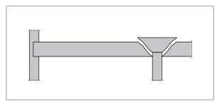
Fig. 1: punching shear situation
