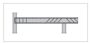
Fig. 4: flat ceiling with stirrups and bent-up rebar
