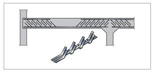
Fig. 3: "Kahn" steel reinforcement system
