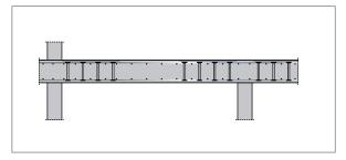
Fig. 5:  $\mathsf{JORDAHL}^{\otimes}$  punching shear reinforcement JDA with double-headed anchors
