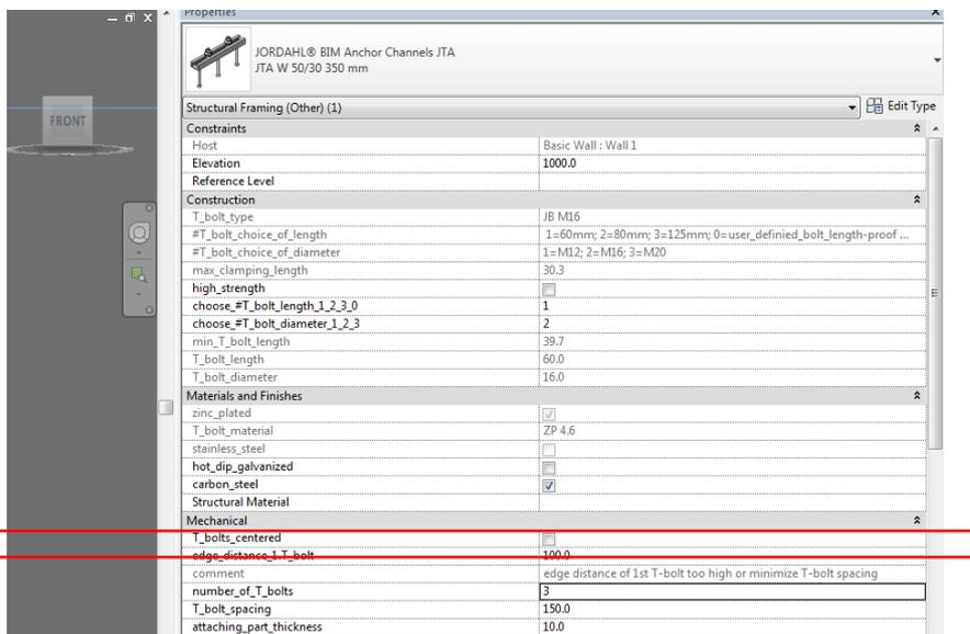
In the above example the selected parameters “edge\_distance\_1.T\_bolt” = 100mm; “number\_of\_T-Bolts”= 3; “T\_Bolt\_spacing”= 150mm for the selected anchor channel JTA W50/30 350mm are not possible, as shown in the highlighted comment. The user might decide to solve this problem by reducing the “edge\_distance\_1.T\_bolt” parameter, or reducing the T-bolt spacing, or selecting a longer anchor channel.
