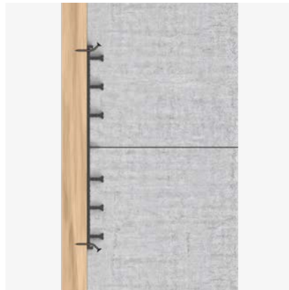
Wall/wall construction joint: Fixed to the formwork.
