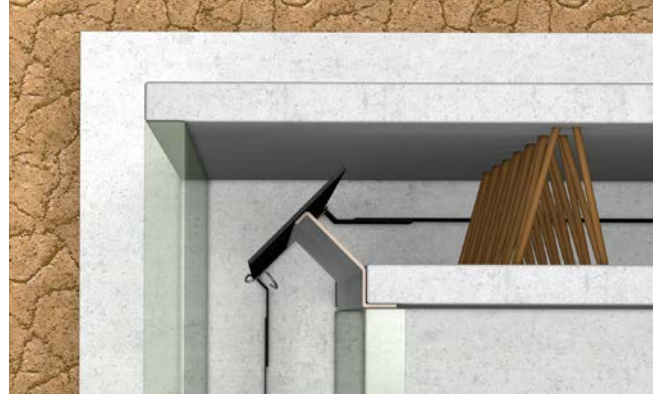
Fig. 2: FTS-Corner for corner joints
