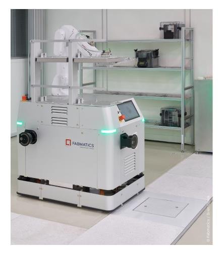
The Dresden-based company Fabmatics specializes in the automation of handling, transport and storage processes in semiconductor factories. Everything revolves around the safe, precise and particle-free handling of high-value wafers, the silicon wafers on which microchips are manufactured. To implement this challenging transport task, Fabmatics has developed, among other things, the HERO®FAB mobile robot.
