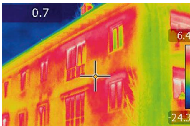
Visualisation of thermal bridges by means of thermography
