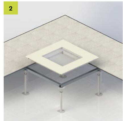
2 Installation of the WCPS raised floor onto the existing supporting structure.
