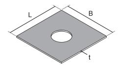
UEBDME V components are square cover inserts. These accessories are used as filling pieces to reduce the floor covering insertion depth in stainless steel tube outlet cartridges, which can be equipped with up to three mounting boxes. The white cover inserts from the range of installation units for underfloor systems are made from high-quality polyvinyl chloride hard foam and have a round outlet for tube units. They are 245 mm across and are made from material 6.0 mm thick.
