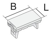
UAA B 22 W components are snap-in covers from the range of installation devices for underfloor systems. These half-size, one-piece plates are used to cover existing cover plates that are used for installation devices are used for installation devices with the dimensions 45x22 mm. The UAA B 22 W are made of high-quality polycarbonate in white.
